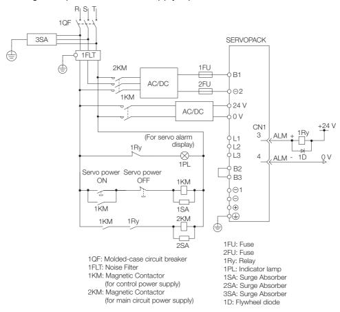
4.3.4 Power Supply Wiring Diagrams
