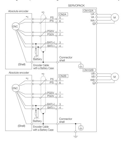
\*1. The absolute encoder pin numbers for wiring the connector depend on the Servomotor that you use.
