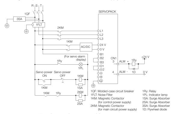
• Wiring Example for DC Power Supply Input: SGD7W-2R6D and -5R4D
